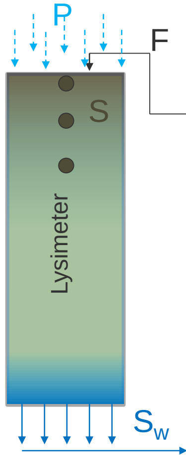
Abb. 10: Sampling strategy to investigate the N-dynamics and N sources of the nitrate in the seepage water. Samples of the atmospheric deposition were taken as well as fertilizer and soil samples, along with four water samples from the recharge at the lysimeter bottom.
